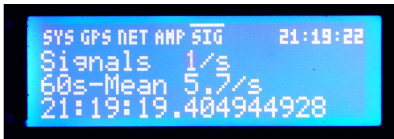
Figure 56: The blue LCD showing the signal page
