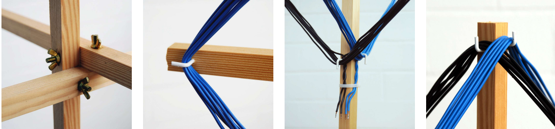
Figure 15: Assembling details for the frame antenna
